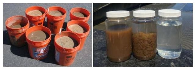
Figure 3. At left, several samples of material for testing. The image on the right shows a raw sample (jar at left) followed by flocculation after polymer addition, and a sample of the filtrate from the Geotube.
