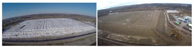
Figure 11. The Geotube dewatering cell at Onondaga Lake is stacked up to five layers high and occupies about 22 hectares. The image on the right shows the cell once capping was complete and prior to adding vegetation.
