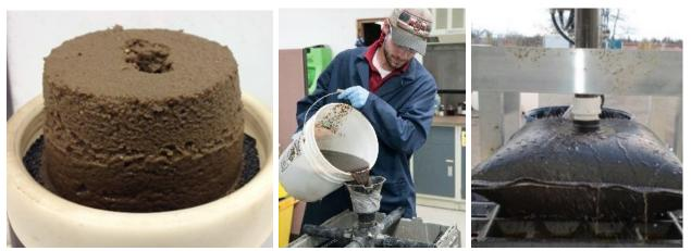
Figure 4. A sludge cake produced by the RDT (left). A technician pours slurry into a GDT container.
