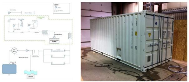
Figure 8. A diagram of the water treatment system (left) and the 6 m container that housed the components.
