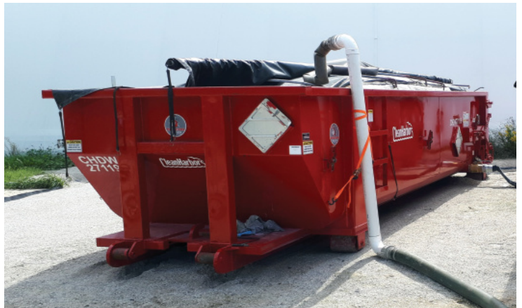
Geotube® containers can be placed in roll-off bins to make removal of dewatered solids fast and easy.
