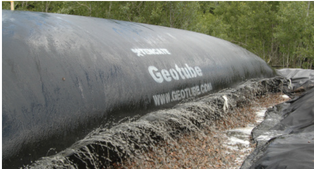
The combination of polymer and Geotube® filtration produces high quality water that may be suitable for discharge or non-potable reuse.
