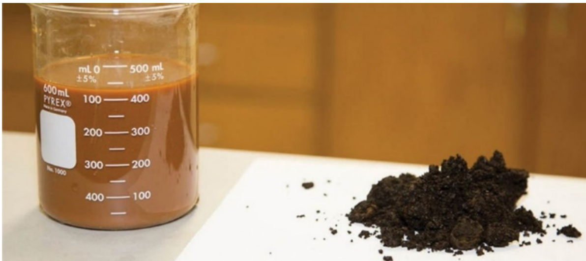
Figure 6. A comparison of the clarifier slurry at 2% solids (left) and the dry solids at 65% from the Geotube dewatering process at the Omega Mine.
