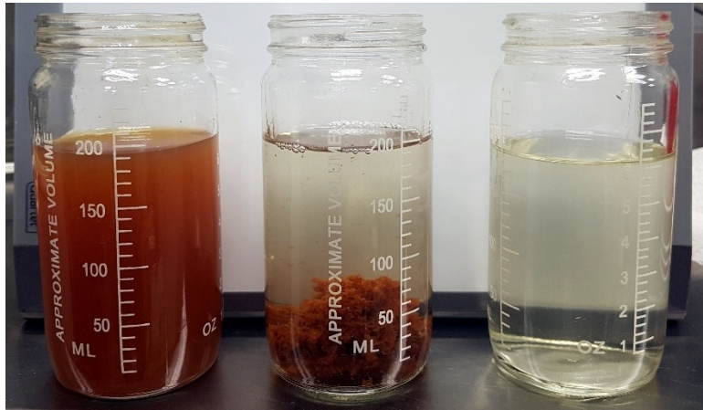
Figure 11. Jar testing shows the results of the process. From left: A sample of the sludge backwash from the MF system; solids clump together after polymer addition; clear filtrate is released from the Geotube container.
