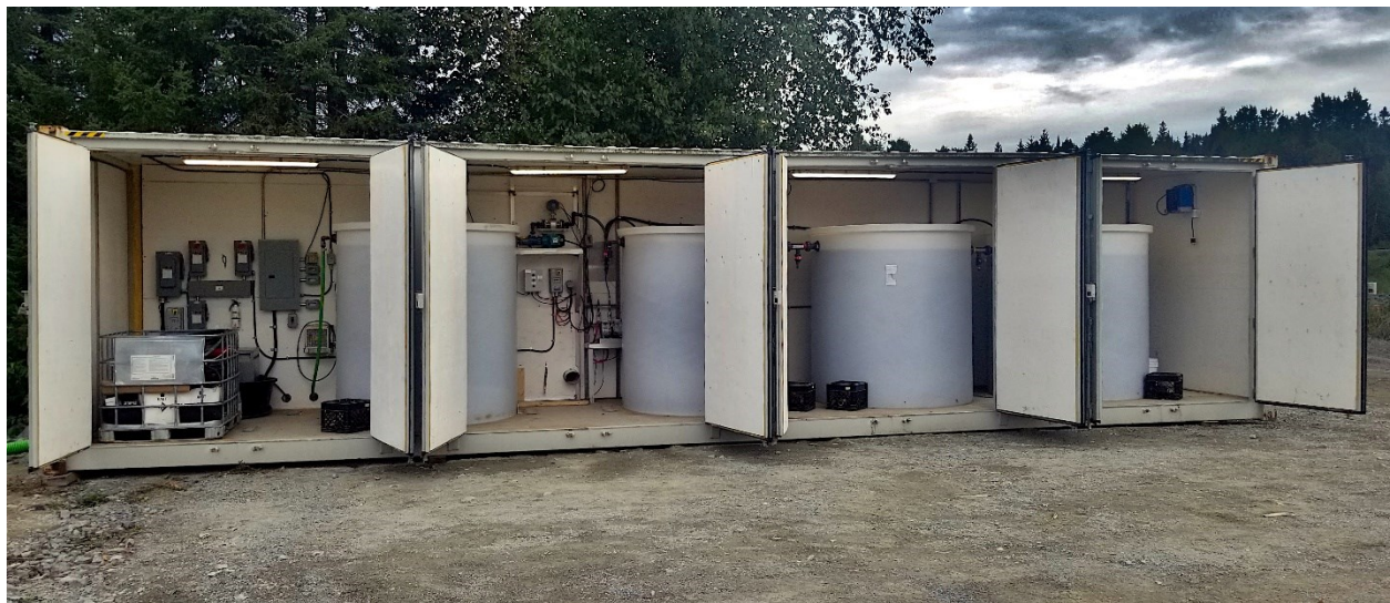
Figure 2. A BioCord Reactor Pilot System equipped with a break tank and three reactor modules.
