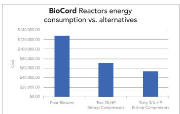
Individual, low-energy compressors supply air to each **BioCord** Reactor, rather than a complex, costly blower. This dramatically reduces electricity requirements for aeration of **BioCord** Reactors compared to systems that use blowers .
