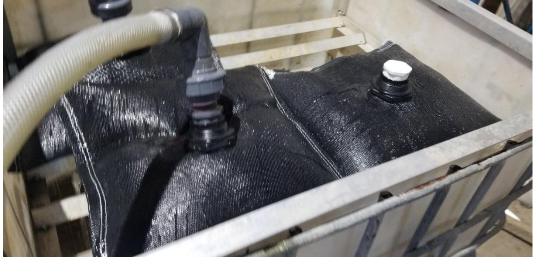
Figure 2. Geotextile dewatering bag for dewatering
