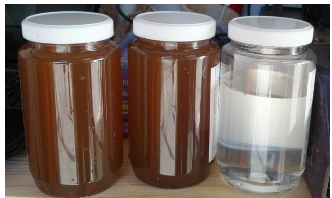
A comparison of the water plant's residual waste stream and the clear filtrate that is released from the Geotube container (right).
