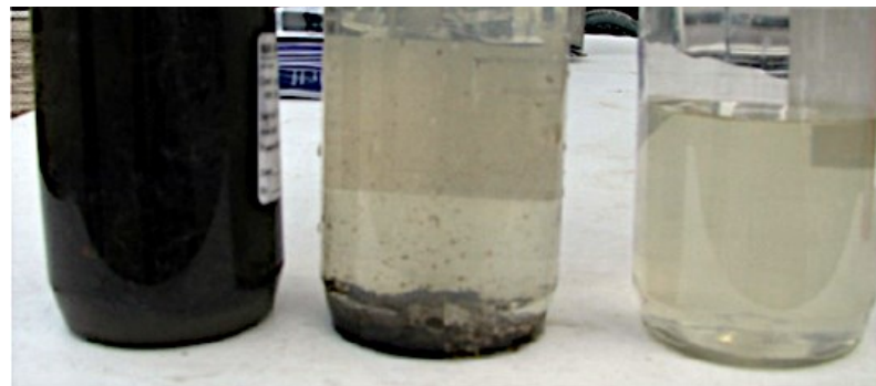
Water samples from the Bishop Solids Management Solution show raw wash water (left), one minute after the addition of coagulant (centre) and treated filtrate from the Geotube® container (right.)
