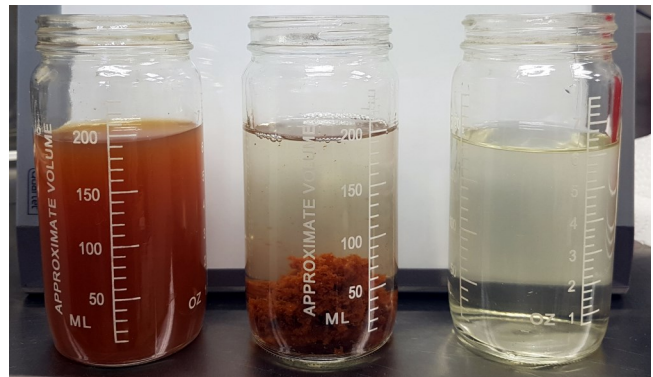
Jar testing shows the results of the simple, low-energy Bishop Solids Management Solution. From left: A sample of the sludge backwash from the MF system; solids clump together after polymer addition; clear filtrate is released from the Geotube container.
