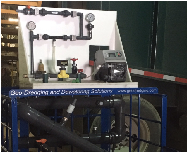
The automated VEPAS eliminates mixers and aging tanks, making the polymer system easy to use and maintain.
