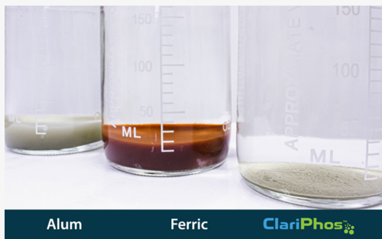
A comparison of sludge produced to remove an equivalent amount of phosphorus.
