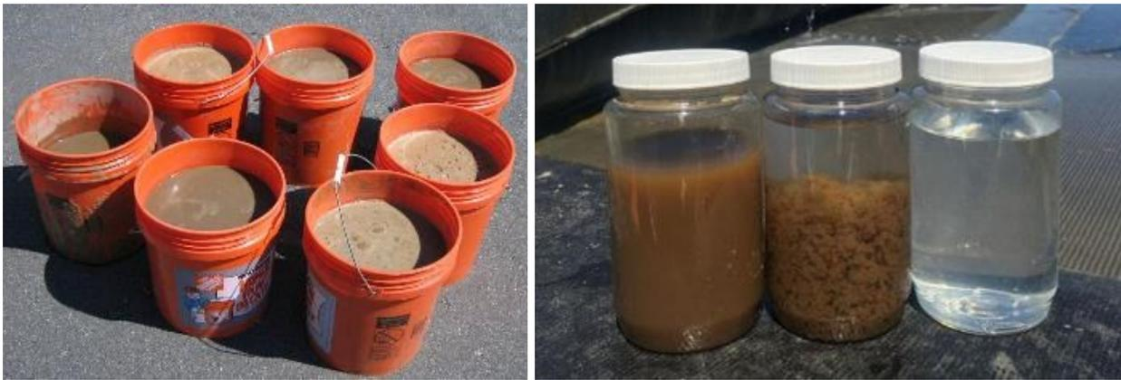
Figure 3. At left, several samples of material for testing. The image on the right shows a raw sample (jar at left) followed by flocculation after polymer addition, and a sample of the filtrate from the Geotube.
