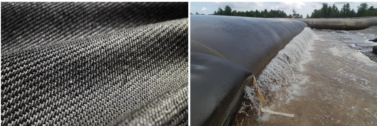
Figure 1. Geotube GT500 material (left) is made from woven polypropylene yarn that provides strong containment and a permeable structure (nominal pore size of 420 $\mu$ m) for rapid dewatering and filtration.
