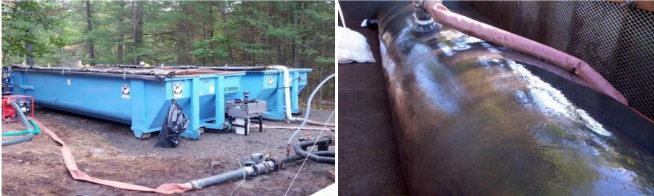
Figure 5. A pilot system was set up to demonstrate onsite polymer conditioning, dewatering and filtration with contaminated sediments as they were removed from the river.
