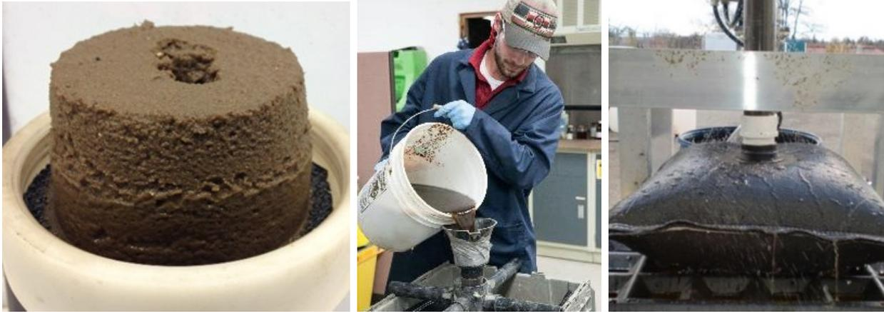
Figure 4. A sludge cake produced by the RDT (left). A technician pours slurry into a GDT container.
