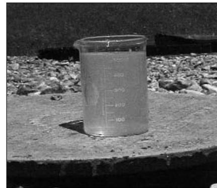
Resulting filtrate weeping out of the Geotube® container at about 8 mg/l permitted the filtrate to discharge directly to the river.
