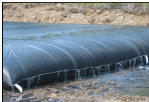
*Clear effluent draining during the initial testing phase.*
