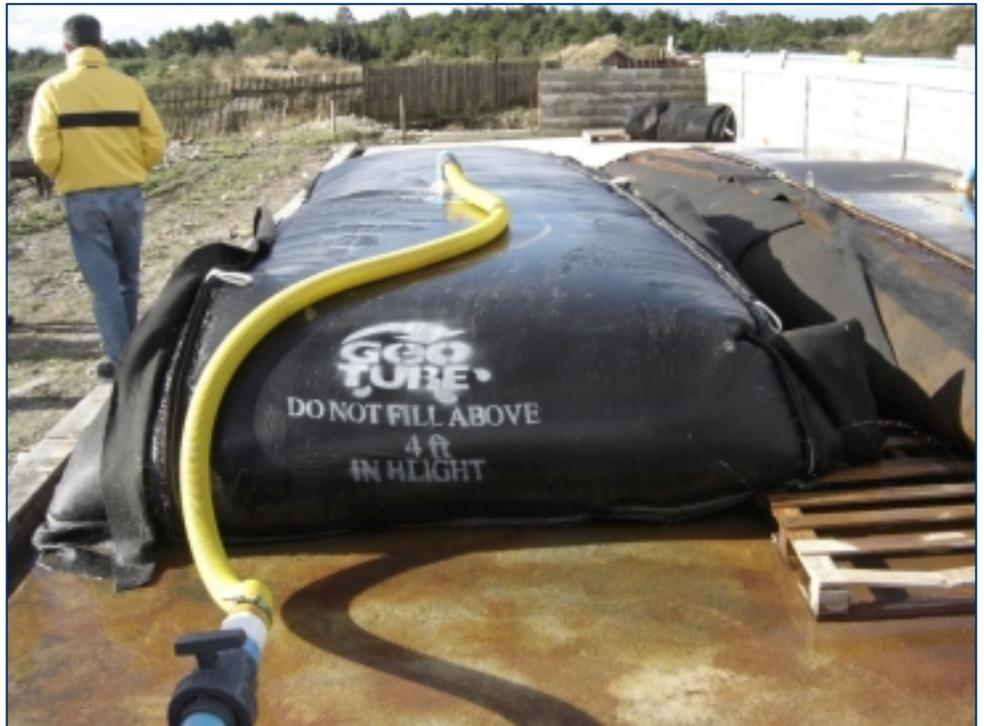
*At this fish processing plant, Geotube® dewatering technology was used to capture wastes in a blood water stream. The Geotube® container captured virtually all of the solids and allowed the facility to return the cleaned water to local streams without further treatment.*
