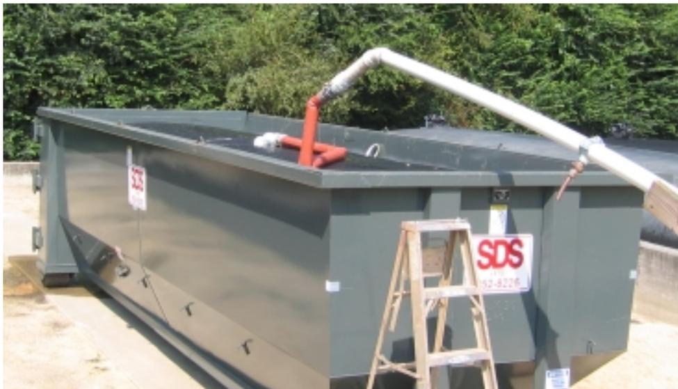
*Geotube® containers are available in a variety of sizes to provide flexible capacity. This one, a Geotube® MDS (mobile dewatering system) container, is in a roll off box for easy removal once dewatering is complete.*
