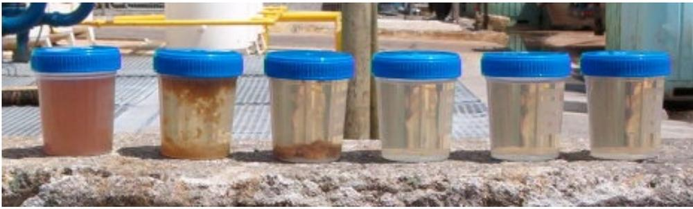
*Polymer added to the waste stream causes solids to bond together for additional dewatering efficiency. After processing through the Geotube® container, the effluent is clear and remarkably clean (right).*
