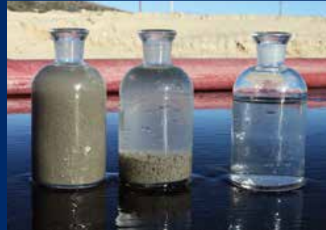
Sludge before (left) and after (right) treatment with Geotube® dewatering technology.
