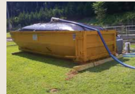
Geotube® Mobile Dewatering System
