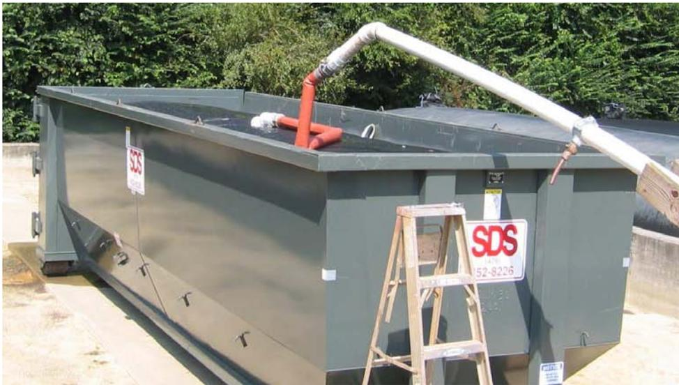
*Geotube® MDS containers fit into a roll-off box for easy removal once dewatering is complete.*
