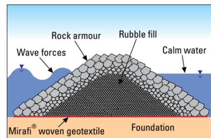
Mirafi® woven geotextile filter placed beneath the rubble breakwater
