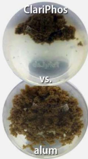
*A comparison of sludge produced to remove an equivalent amount of phosphorus.*
